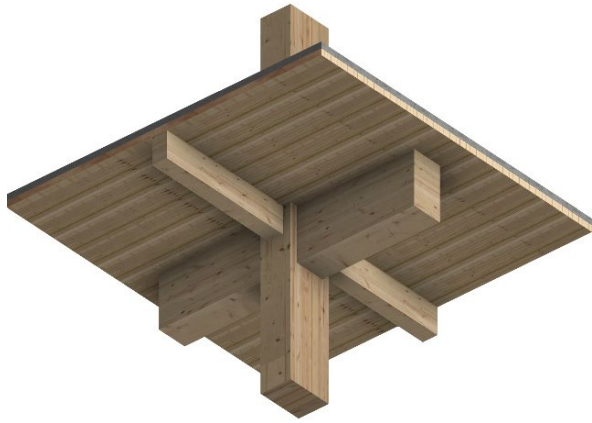
Mass Timber Floor Framing
